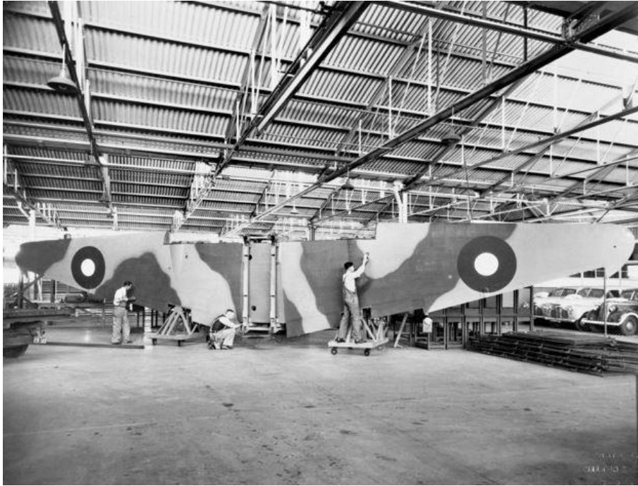
Figure 35 – c1943. Employees of De Havilland Aircraft Pty Ltd at GMH Pagewood NSW painting camouflage colours, one of the final stages of wing assembly for DH98 Mosquitos.
